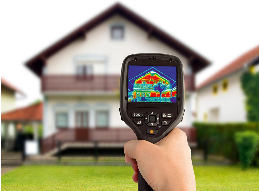
Fig.2 – Example of hand-held IR camera.
